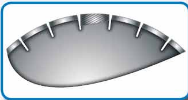
C - A Regular Segment Set on a Slant. Used mainly on regular concrete and asphalt saws. Part of the slanted segment is dedicated for undercutting protection.
